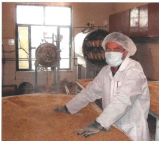
The cooked wheat is placed on tables for the steam to escape before being placed in bags and sterilised.
